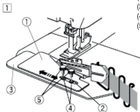
2. Align the folded tape and the needles by sliding the binder to the left or right. Tighten the two thumbscrews securely.
