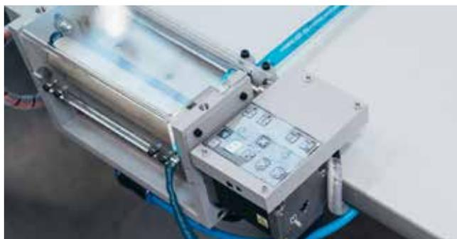
Fig.: Automatic Pull Through Device of ROLL2BASKET
