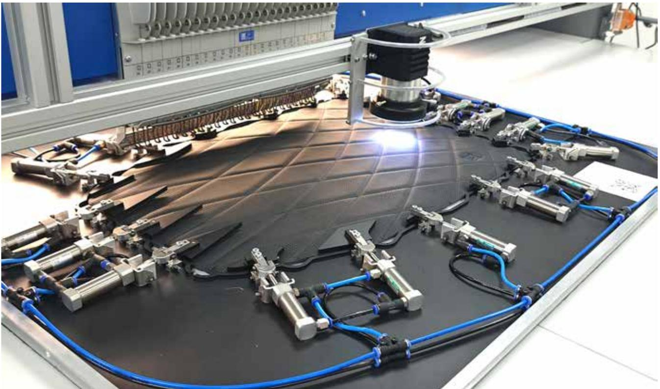
Machine: RACER 0124 with 24 needles and ZSK Vision System.
