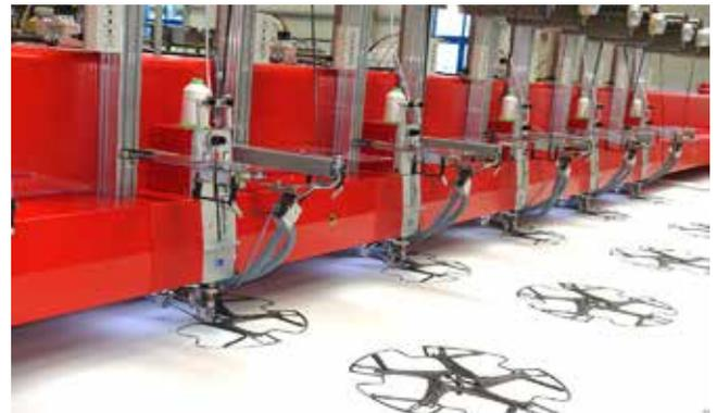
ZSK Technical System CZCW 0809- with eight W-Heads placing and fixing fibers.
