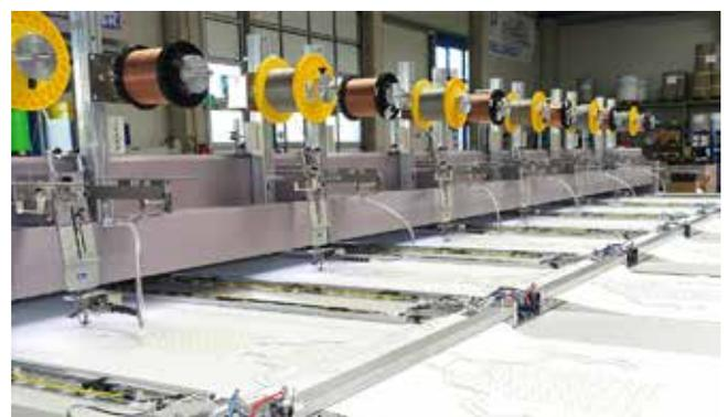
ZSK's Technical System CYCW 0600- placing and fixing conductive thread for automotive heating systems.
